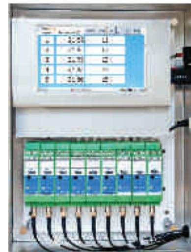
The PowerTemp series is a new multichannel temperature sensor and transmitter for the power and utility industry.
